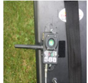
**FOR MAXIMUM ELECTRONIC RANGE:** Mount the receiver so its antenna extends beyond the launcher case. See Photo
