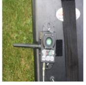
3. MOVE LAUNCHER POWER SWITCH TO "ON" POSITION AND DEPRESS YOUR ELECTRONICS TO ENSURE THE MACHINE CYCLES PROPERLY AND IS IN THE NEUTRAL POSITION (Smaller hole between bumper tubes over firing hole on launcher)
